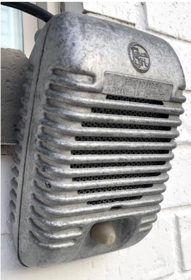
Window speaker from the Tropicaire Drive-in Theatre. Each stand had two speakers, one for each car parked on either side of the stand.
