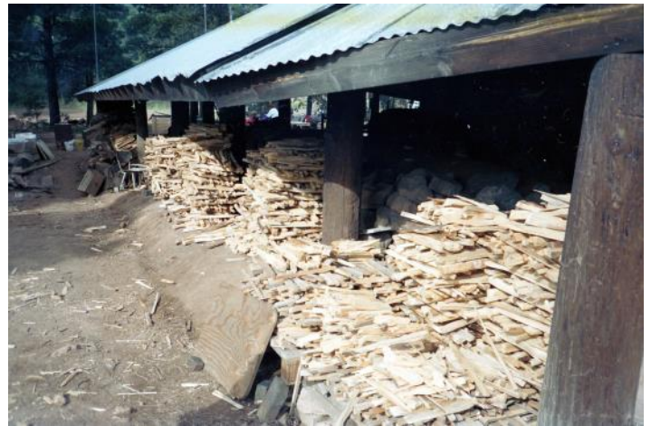
Except for the wood in the front of the kiln, all of the rest of the wood had to be cut down into thin sticks to fit through the side stoke holes on the kiln.
