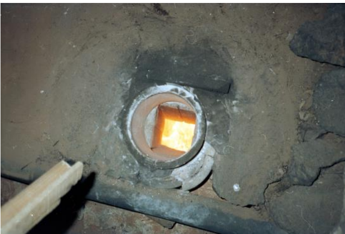
Once the front fire got hot enough, it was sealed and three sets of side holes were fed sticks of wood in regular intervals until the entire kiln got hot enough for all of the pottery to be properly fired. At that
