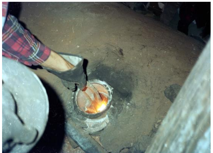
point, all holes were sealed and the entire kiln allowed to cook, which took about a week.
