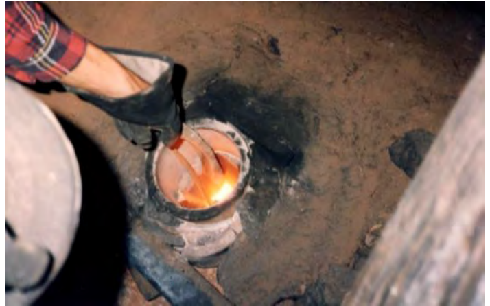
Above and below: Little holes on each side of the kiln allow for the dropping in of wood. The wood keeps the fire going as well as provides for the wood to burn, creating ash which then melts on the pottery as a glaze. As you can see, the kiln gets to a yellow glowing hot and stays that way for a few days until the temp gets to the point where the pottery itself can start to melt!
