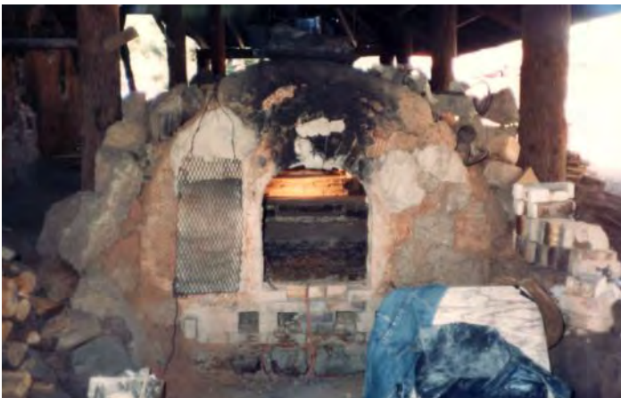
Below: The firing of the Anagama kiln takes several days and requires a lot of wood, and specifically in little sticks to fit through the small holes on each side of the kiln.
