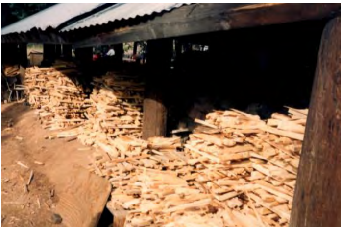
Below: The firing of the Anagama kiln takes several days and requires a lot of wood, and specifically in little sticks to fit through the small holes on each side of the kiln.
