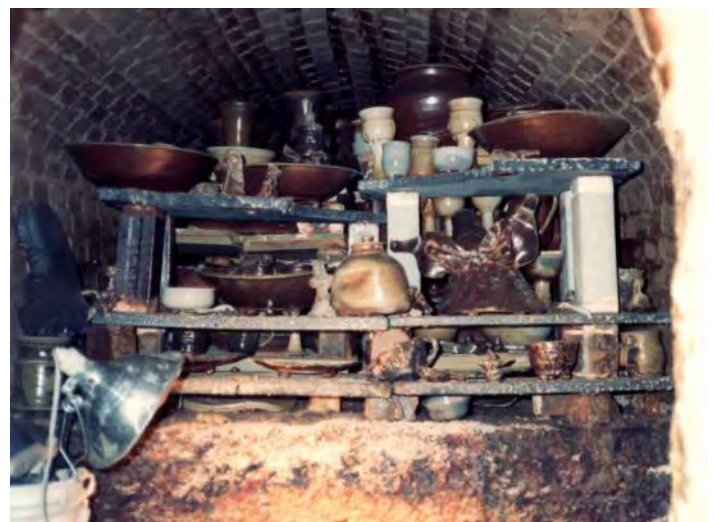
Above: Once the kiln is hot enough, no more wood is added and all openings are sealed up with bricks and/or clay. The kiln then slowly cools to room temp, which takes several days. The pottery will still be rather hot, but cool enough to touch. The pottery inherently gets a range of browns caused by the fire and the ash glaze (besides any glazes put on the pottery beforehand).
