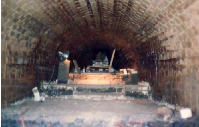
Above: This is the inside of the Anagama kiln before loading it. Below: This is the front of the Anagama kiln.
