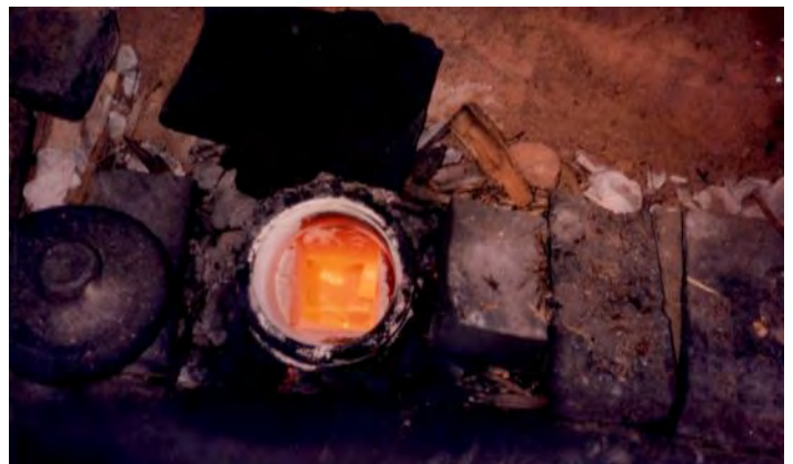
Above and below: Little holes on each side of the kiln allow for the dropping in of wood. The wood keeps the fire going as well as provides for the wood to burn, creating ash which then melts on the pottery as a glaze. As you can see, the kiln gets to a yellow glowing hot and stays that way for a few days until the temp gets to the point where the pottery itself can start to melt!
