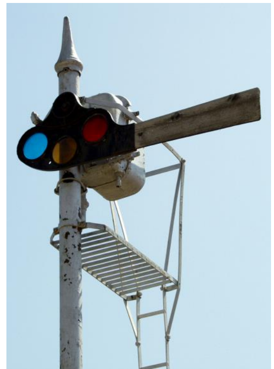
Left: This is the station signal on the Ropes Depot at the NRHC. You can see where the lamp would sit at the top on a bracket.
