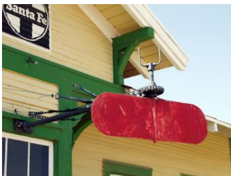
Left: This is the station signal on the Ropes Depot at the NRHC. You can see where the lamp would sit at the top on a bracket.
