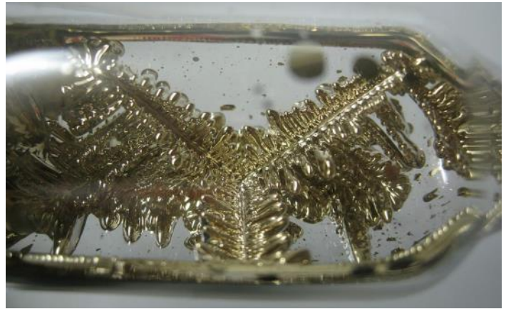
High purity cesium-133 stored in the inert gas argon. Cesium is highly reactive and ignites spontaneously in air and reacts explosively with any temperature of water.
